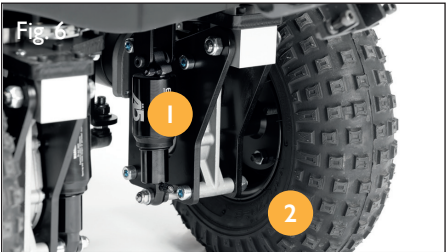
1. Principale MP pressure valve 2. Secondary MP pressure valve
