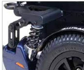
Interactive suspension for the 6 wheels and the seat provide greater stability, mobility and comfort.
