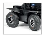
Equipped with 4 350W motorised wheels, can obtain 10 km/h.
