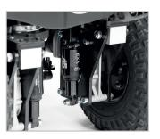
Its two air shock-absorbers are adjustable and adapt the suspension depending on the user's needs.
