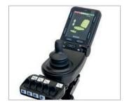
CISM2 Joystick and keyboard (optional) to facilitate driving and secure the use of different positions.
