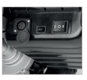
Battery charging and folding/unfolding switches.
