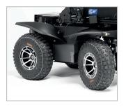
Equipped with 4 350W motorised wheels, can obtain 10 km/h.
