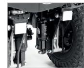
Its two air shock-absorbers are adjustable and adapt the suspension depending on the user's needs.
