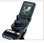
CJSM2 Joystick and keyboard (optional) to facilitate driving and secure the use of different positions.
