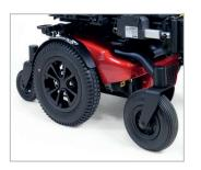
Hybrid configuration which combines the characteristics of median traction and rear wheel propulsion.
