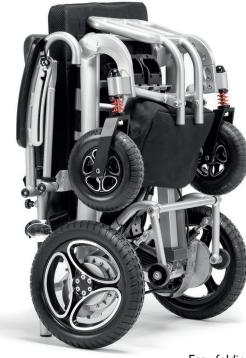
Easy folding and unfolding for storage and transporting in the boot of a vehicle.
